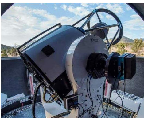
Many key features of large mountaintop research telescope, such as alt-az mounts, dual Nasmyth foci, direct drives, and advanced optics, that were captured by the Alt-Az Initiative community of practice have been incorporated in production-line telescopes built by PlaneWave Instruments. Left: 0.7-meter telescope at the Great Basin Observatory. Right: the 1.0-meter telescope and undergraduate student researchers at the College of the Desert.
