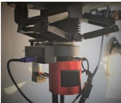
Figure 2: The instrument cluster includes a Clement focuser, a ZWO filter wheel, and CMOS camera.
