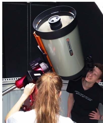
The 14-inch Celestron Schmidt-Cassegrain telescope at Concordia University will use a high speed camera to overcome seeing limitations and make speckle interferometry observations of close binary stars.
